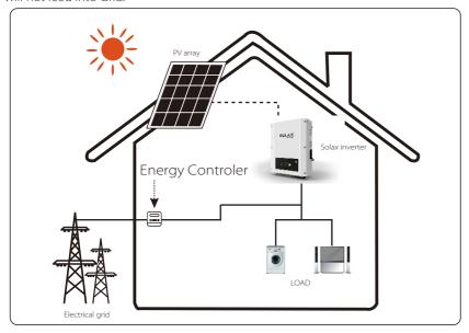
Wherever you use the Energy Controler, first you need confirm it can be communicate with the inverter. It is compatible with Solax inverter:
